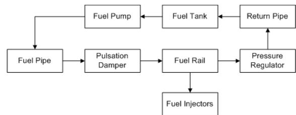
Fig. 1 Fuel Delivery System Block Diagram
