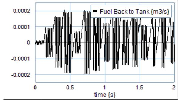
Fig. 22 97% Model Pressure Regulator Output Fuel Flow Transient Response
