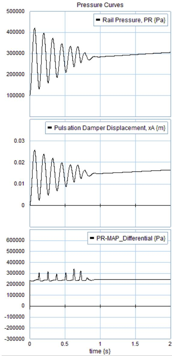
Fig. 19 98% Model Transient Pressure Responses
