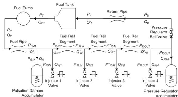
Fig. 2 Fuel Delivery System Schematic
