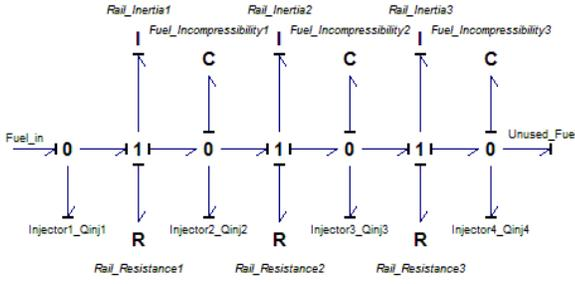
Fig. 7 Fuel Rail Submodel
