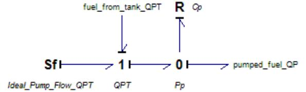
Fig. 4 Fuel Pump Submodel
