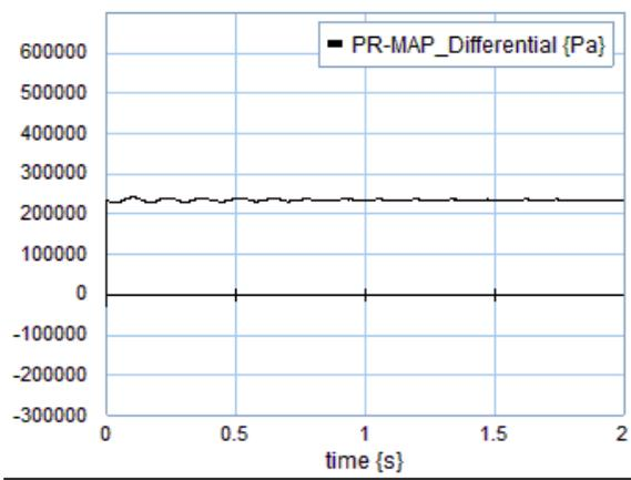
Fig. 21 97% Model Rail Pressure Differential Transient Response
