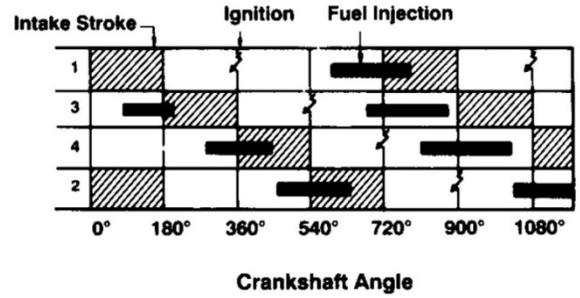
Fig. 8 Sequential Fuel Injection (SFI) Pattern [4]
