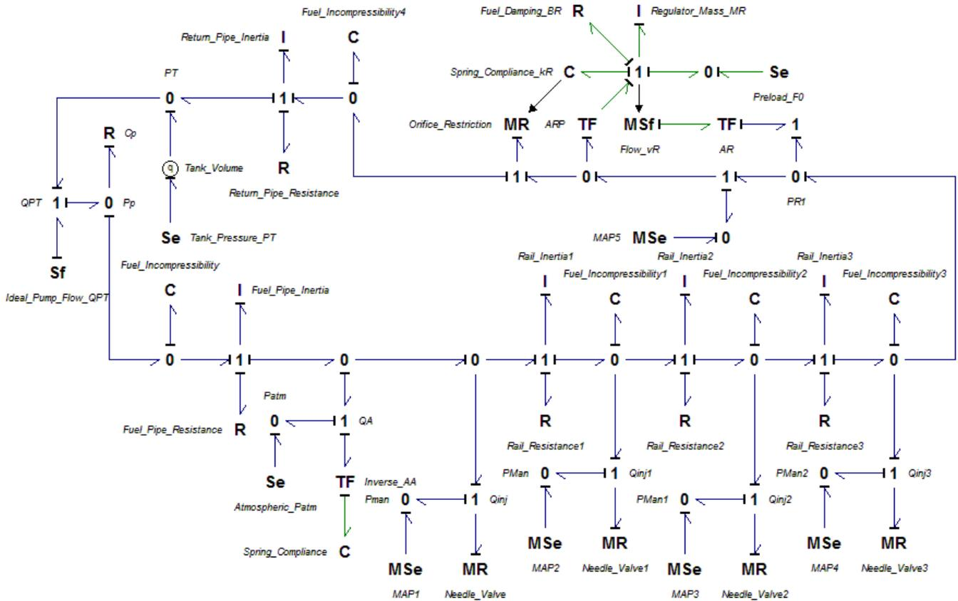
Fig. 11 Fuel Delivery System Complete Model
