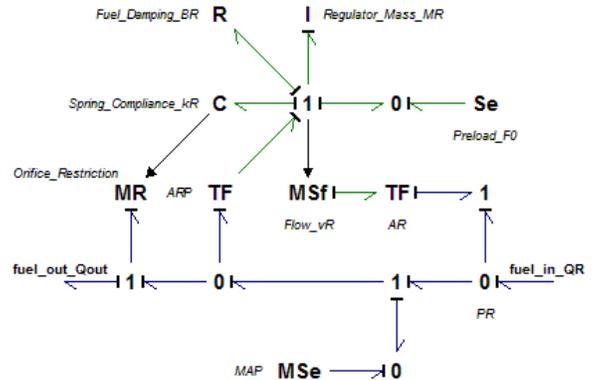
Fig. 10 Fuel Pressure Regulator Submodel
