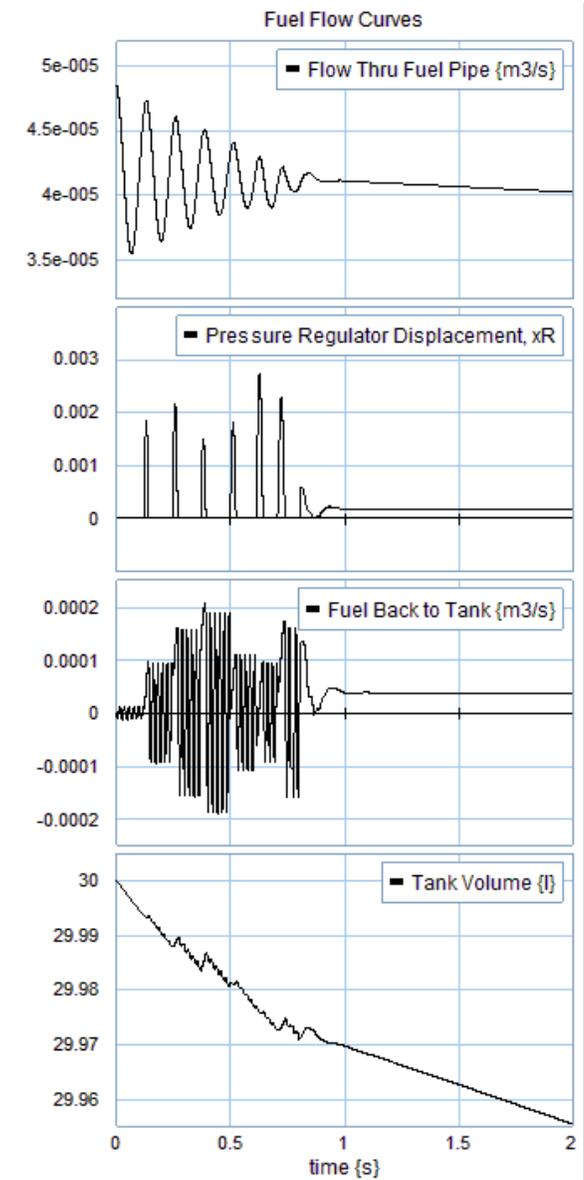
Fig. 20 98% Model Transient Flow Responses
