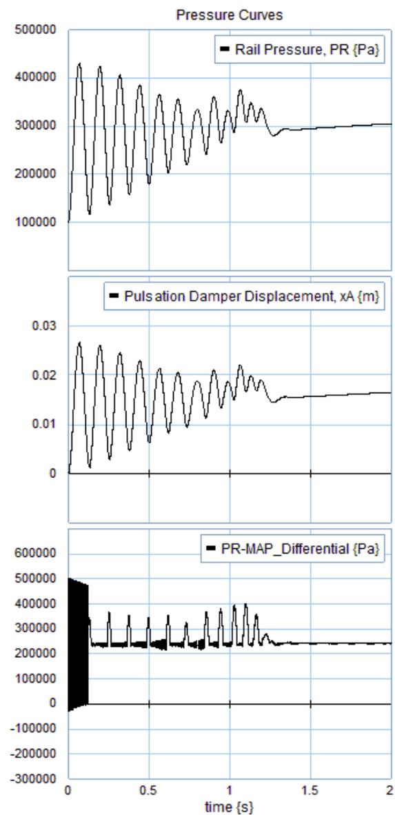
Fig. 17 99% Model Transient Pressure Responses
