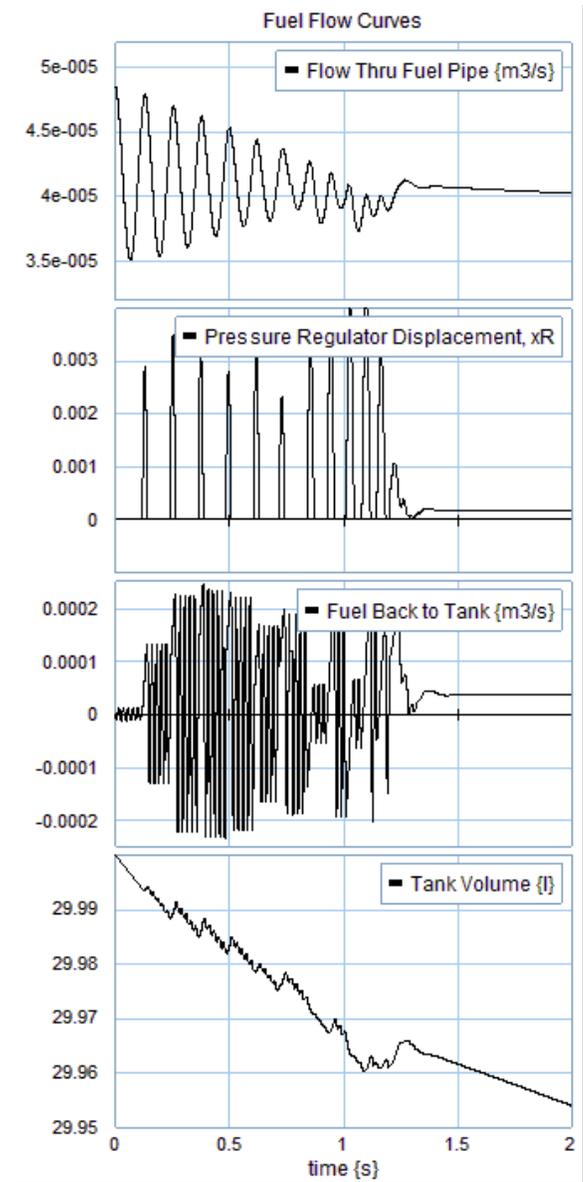
Fig. 18 99% Model Transient Flow Responses
