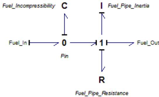
Fig. 5 Fuel Pipe Submodel
